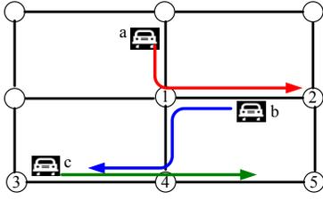
Fig. 1. Data forwarding through predicted encountered vehicles
