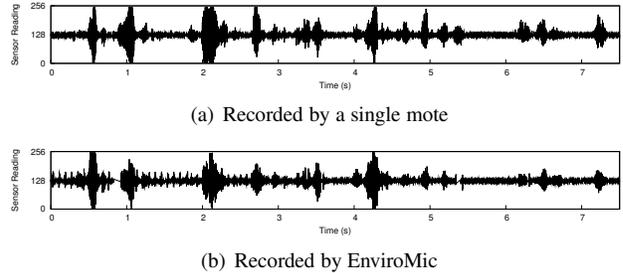
Figure 4: Recording voice of a moving human being
